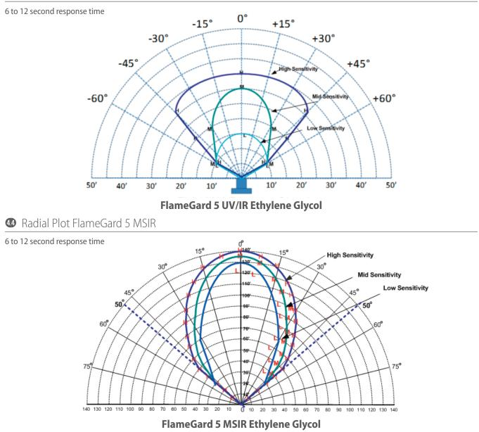
Note: FlameGard 5 MSIR can have up to 60 degree Field of View at 125' with longer response time (12 to 25 seconds).
