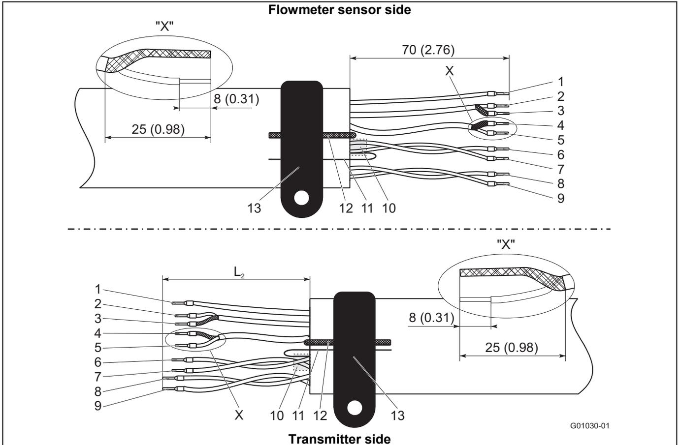
Fig. 36: Flowmeter sensor side, dimensions in mm (inch)
