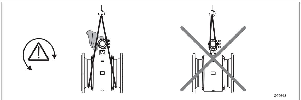
Fig. 9: Transport of flanged units smaller than DN 450
