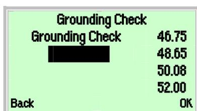
Once the grounding check has been started, the frequency range up to 250 Hz is measured. The four most intensive frequencies of the spectrum are shown at the right of the display.
