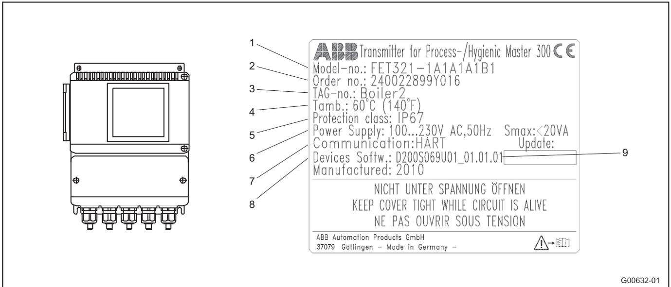
Fig. 3: External transmitter (e.g., transmitter with dual-compartment housing)
