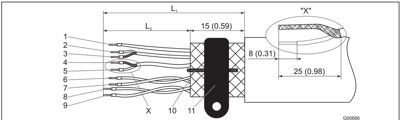
Fig. 35: Transmitter side, dimensions in mm (inch)
