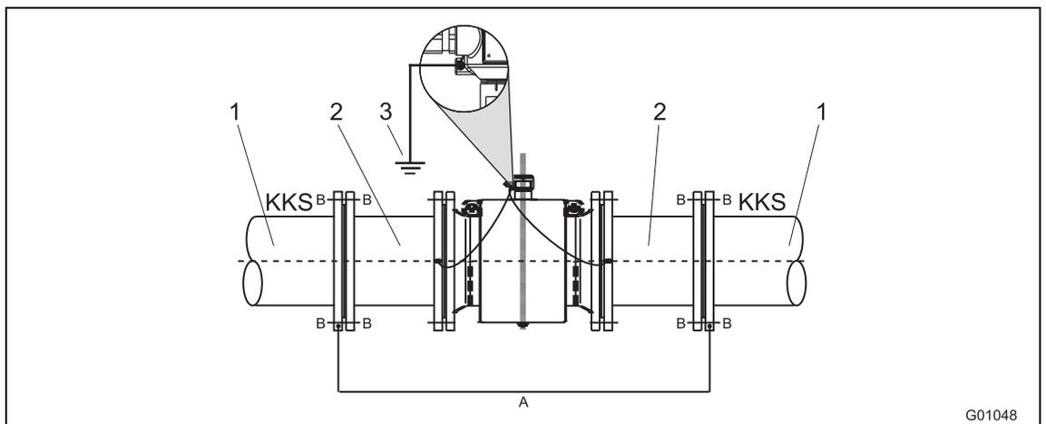
Fig. 32: Flowmeter sensor with functional ground
