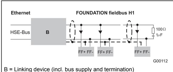
Fig. 57: Example for FOUNDATION fieldbus interface connection
