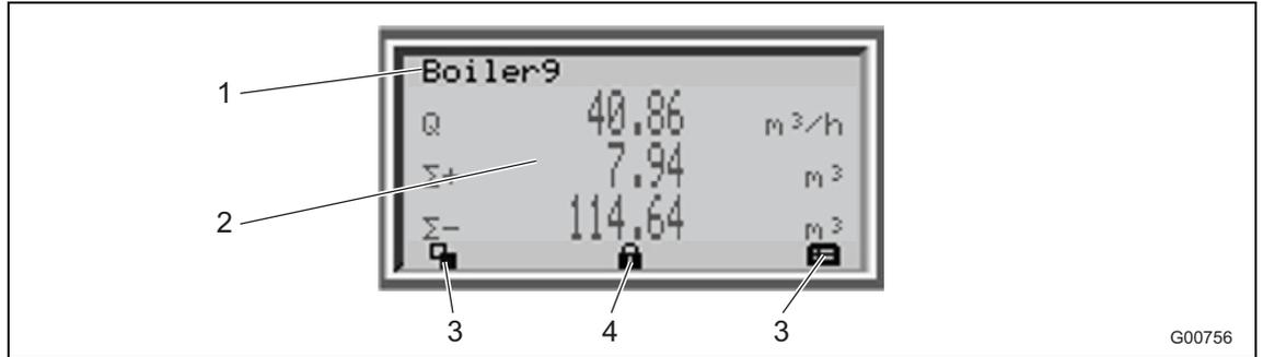
Fig. 66: Process display (example)
