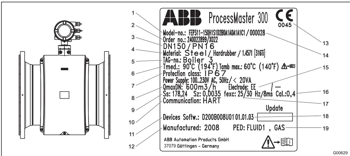
Fig. 1: Compact device (e.g., transmitter with dual-compartment housing)
