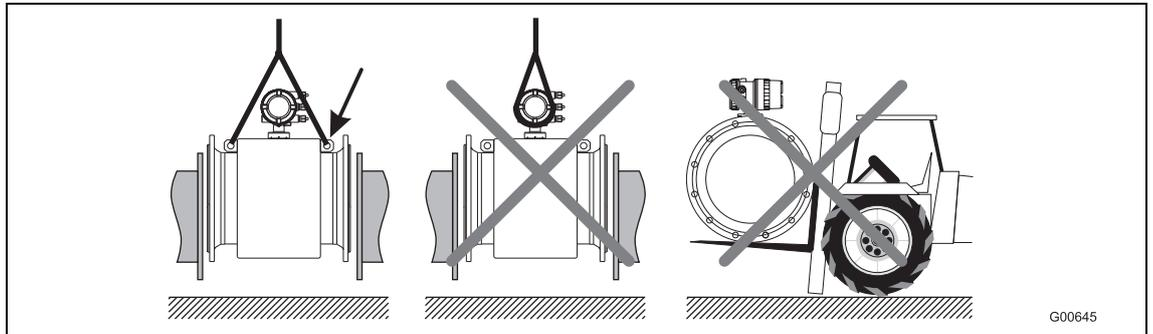
Fig. 10: Transport of flanged units larger than DN 400
