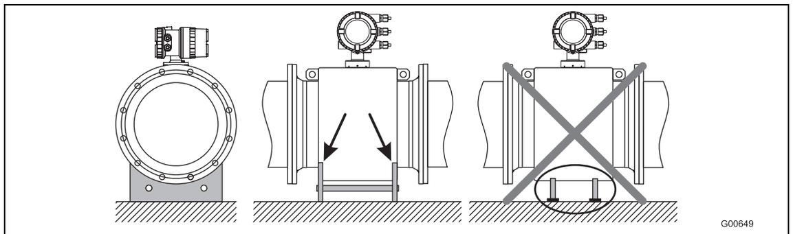
Fig. 11: Support for meter sizes larger than DN 400
