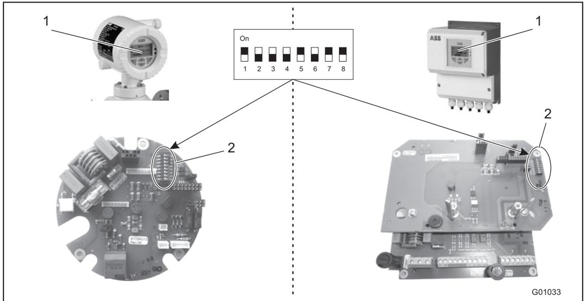
Fig. 62: Position of DIP switches
