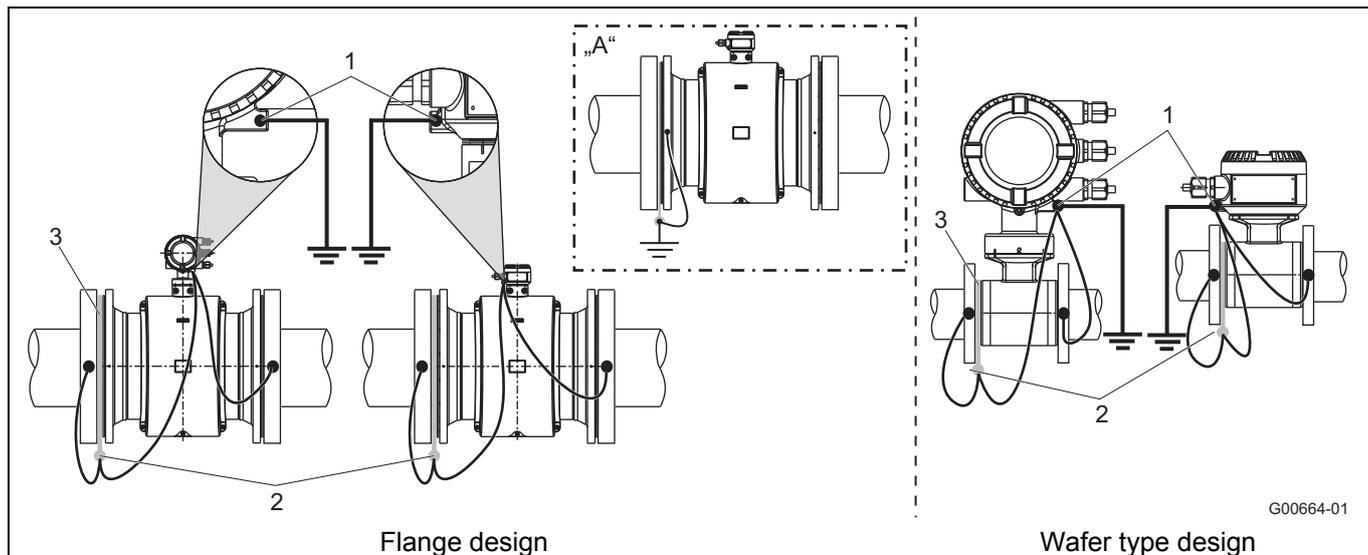
Fig. 28: Plastic pipes, non-metallic pipes or pipes with insulating lining
