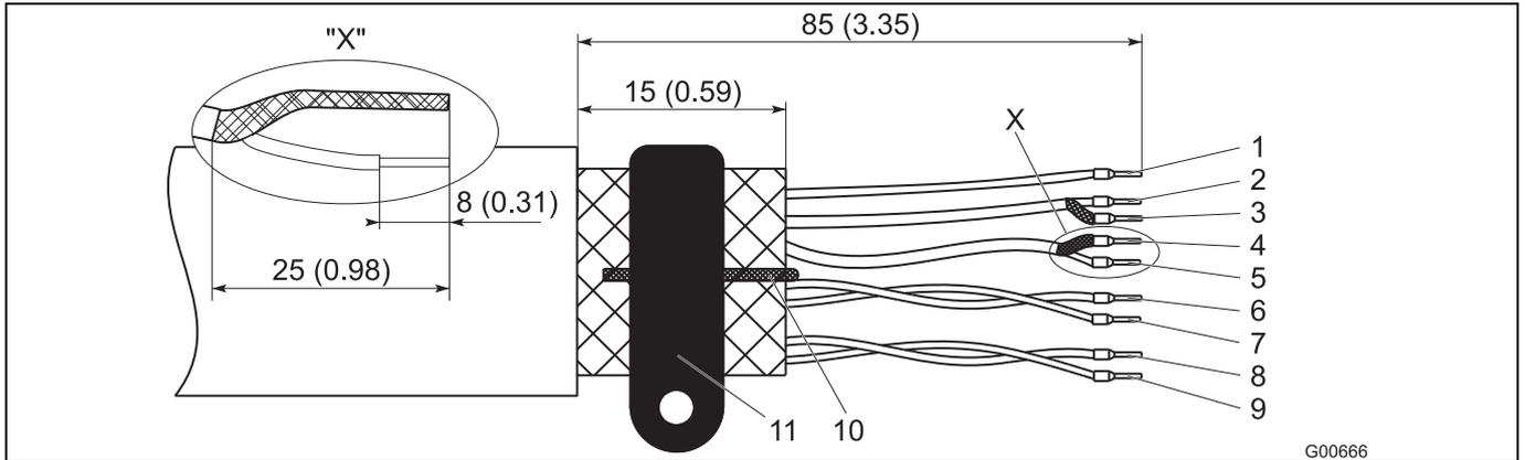
Fig. 34: Flowmeter sensor side, dimensions in mm (inch)
