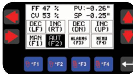
The control screen displays the relationships between stack draft and set point, feedforward variable and damper. Also, controls set point adjustment, select auto or manual mode; and increase/ decrease the output to the outlet damper.
