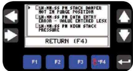
The alarm history shows all acknowledged and unacknowledged alarms with time stamp. Alarms include High Stack Pressure and Stack Damper not In Purge Position.
