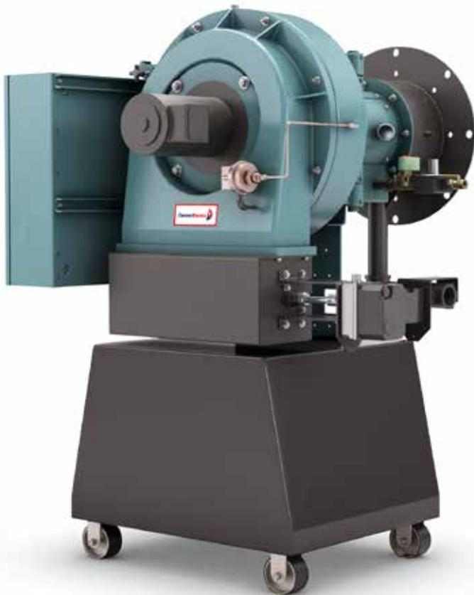
**Low-pressure** air atomizing system on oil with rotary vane compressor purges air through the large nozzle orifice after each burner cycle to prevent after-drip and fouling.
