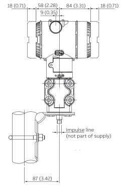
Figure 2 Standard static transmitter with barrel housing - vertical flanges
