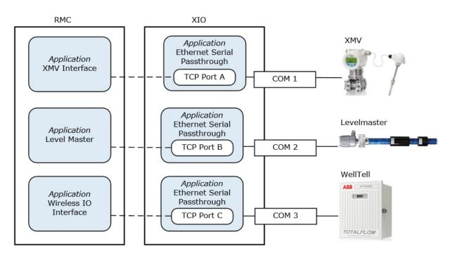
The connection between each communication application and its corresponding remote device is client-server based. The communication application on the RMC performs the client role and the Ethernet-Serial passthrough on the XIO performs the server role. As clients, the communication applications initiate connection requests to the passthrough instances. Once connection is successfully established, the application interacts with the device as designed for the device type.
