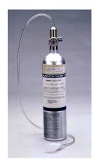
Figure 21: Portable Purge Calibrator
