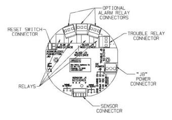
Figure A-2. Relay Printed Circuit Board
