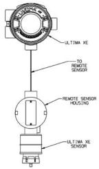
Figure 1-19. Remote Module Explosion-Proof Ultima X Series Wiring
