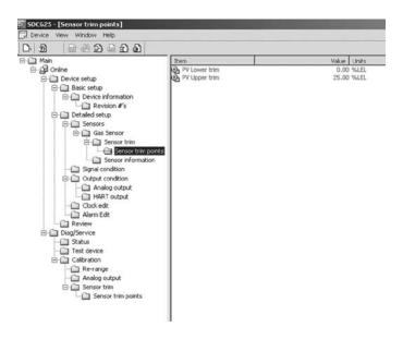
Figure D-17. Sensor Trim Point screen
