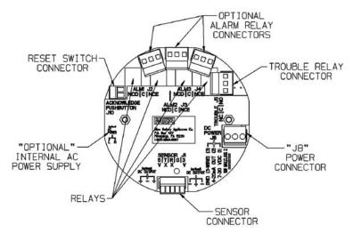
Figure 1-16. Three-Wire Printed Circuit Board (no HART Protocol)
