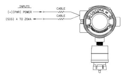
Figure 1-11. Explosion-Proof Two-Wire Operation
