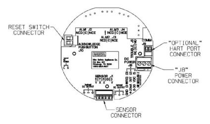
Figure 1-15. Two-Wire Printed Circuit Board (with HART Protocol)
