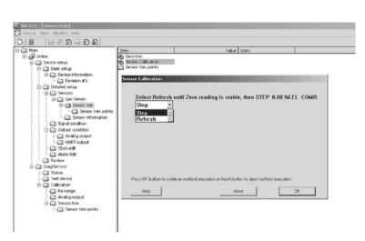
Figure D-1. Zero cal step screen
