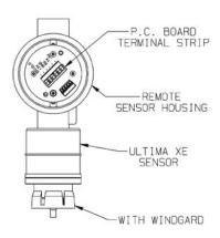
Figure 1-5. Explosion-Proof XE Remote Sensor Module
