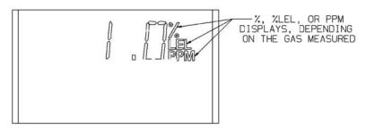
Figure 2-1. LCD Gas Concentration Display
