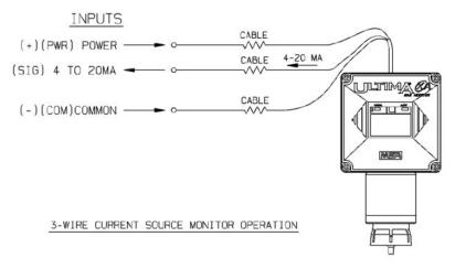
Figure 1-12. General-Purpose Three-Wire Operation
