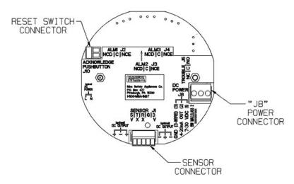
Figure 1-14. Two-Wire Printed Circuit Board (no HART Protocol)
