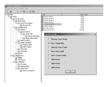
Figure D-18. Additional Sensor Status screen
