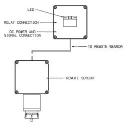
Figure 1-18. Remote Module General-Purpose Ultima X Series Wiring
