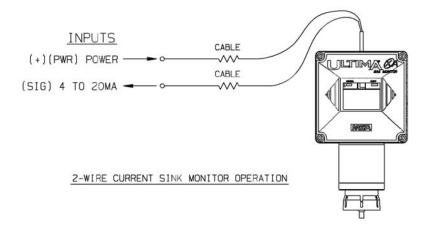
Figure 1-10. General-Purpose Two-Wire Operation
