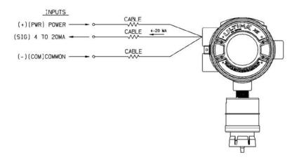
Figure 1-13. Explosion-Proof Three-Wire Operation
