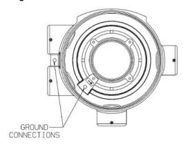
Figure 1-9. Ultima XE Grounding Terminals
