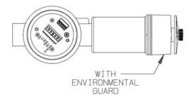
Figure 1-6. Explosion-Proof XIR Remote Sensor Module
