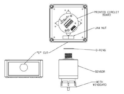
Figure 1-4. General-Purpose XA Remote Sensor Module
