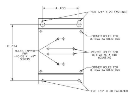
Figure 1-7. Ultima XE and XIR Mounting Bracket
