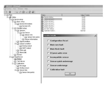
Figure D-19. Device Status screen
