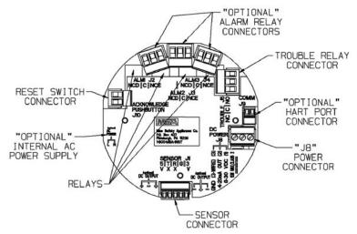
Figure 1-17. Three-Wire Printed Circuit Board (with HART Protocol)
