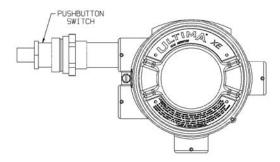
Figure 2-4. Ultima X Optional Push-button Calibrator
