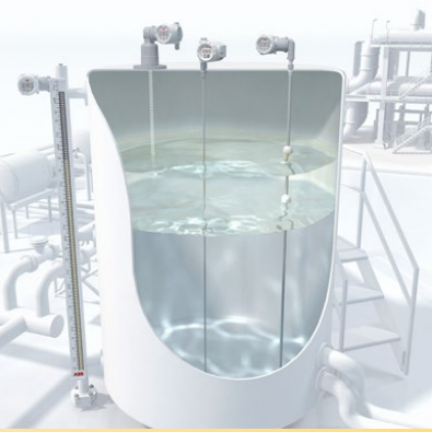
Figure 1: Level Measurement determines the position of the level relative to the top of bottom of the process fluid storage vessel. A variety of technologies can be used, determined by the characteristics of the fluid and its process conditions.
