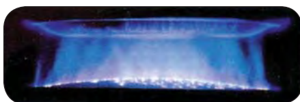
Axial Magnetic Field Interrupter - Arc Dispersion
