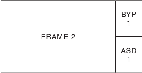
Frame 2 (2250 to 2500 HP): Sync-Xfer Arrangement for Single Motor
