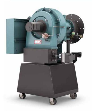
**Low-pressure** air atomizing system on oil with rotary vane compressor purges air through the large nozzle orifice after each burner cycle to prevent after-drip and fouling.
