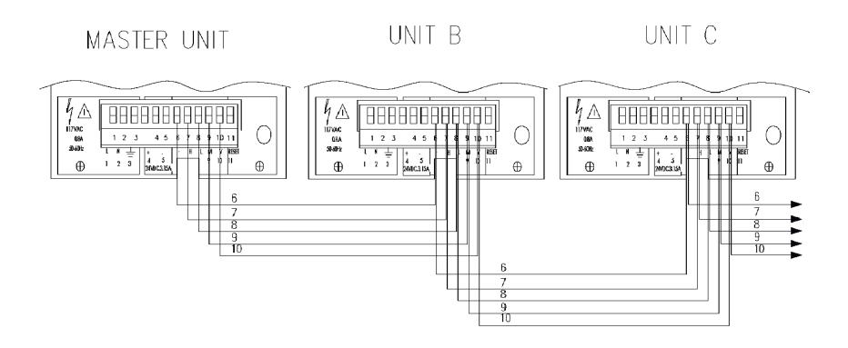
Figure 11: Interconnection Drawing Zone Control Model 610A Controller
