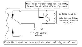
**Figure 7: Protection Circuit for Relay Contacts**
