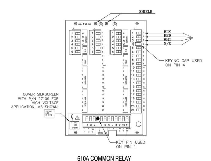
Figure 4: Rear Terminal Common Relay Configuration
