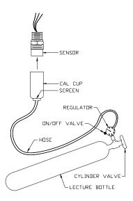
Figure 9: Portable Purge Calibrator
