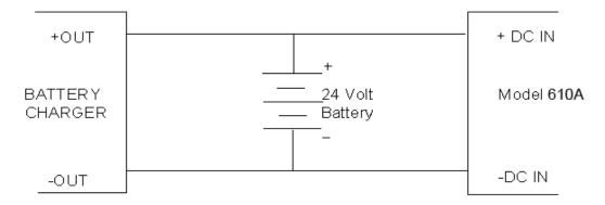
Figure 2: Schematic Battery Backup System
