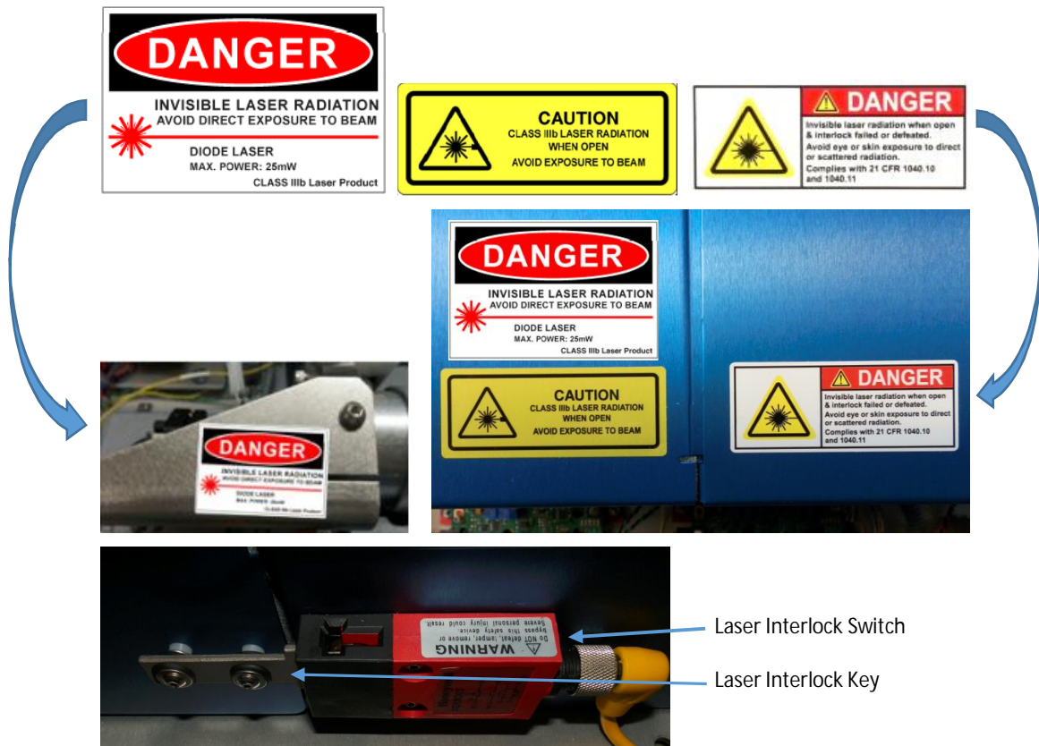
Figure 11 Laser Radiation Labels & Interlock Switch
