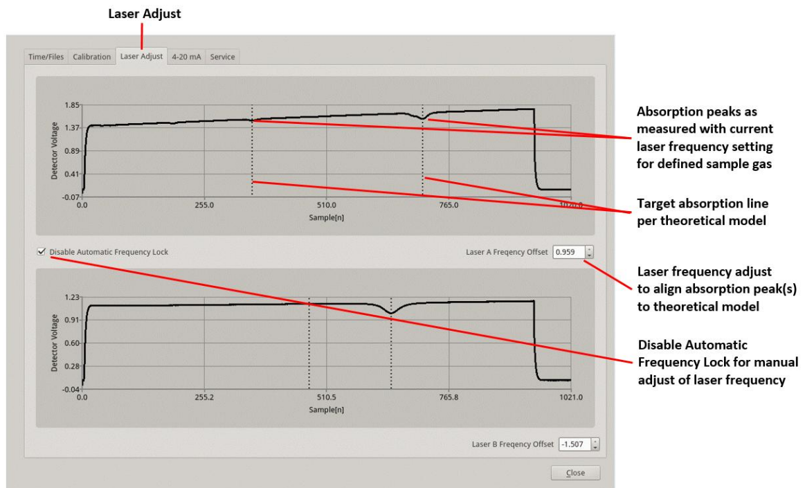
Figure 27 Laser Adjust for Optimizing Measurement Calibration
