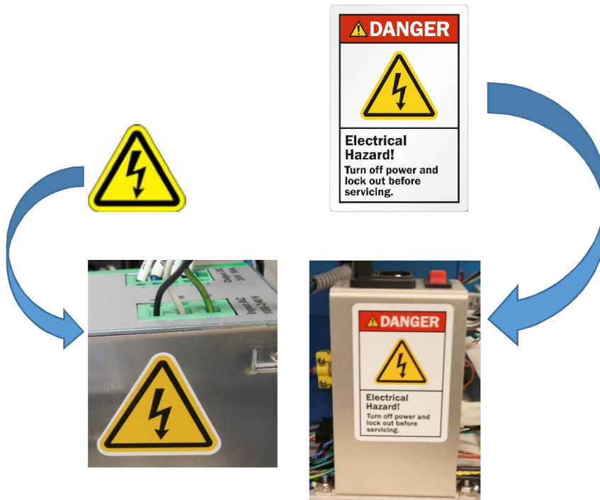
Figure 10 Electrical Hazard Label and Locations
