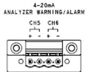
Figure 35 Gas Analyzer Warning/Alarm Phoenix Connection Point
