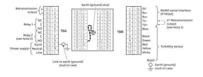
Wall- / Pipe-mount analyzer connections
