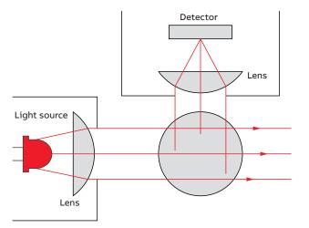
Figure 2 Nephelometric turbidity monitor
