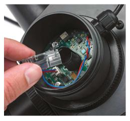
Figure 6 Replacing the light source
