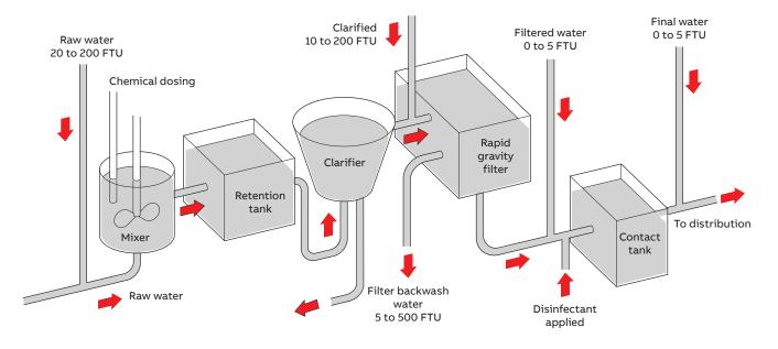
Figure 1 Typical turbidity monitoring application
