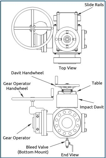
Figure 5: Pig Valve c/w Impact Davit & Gear Operator
