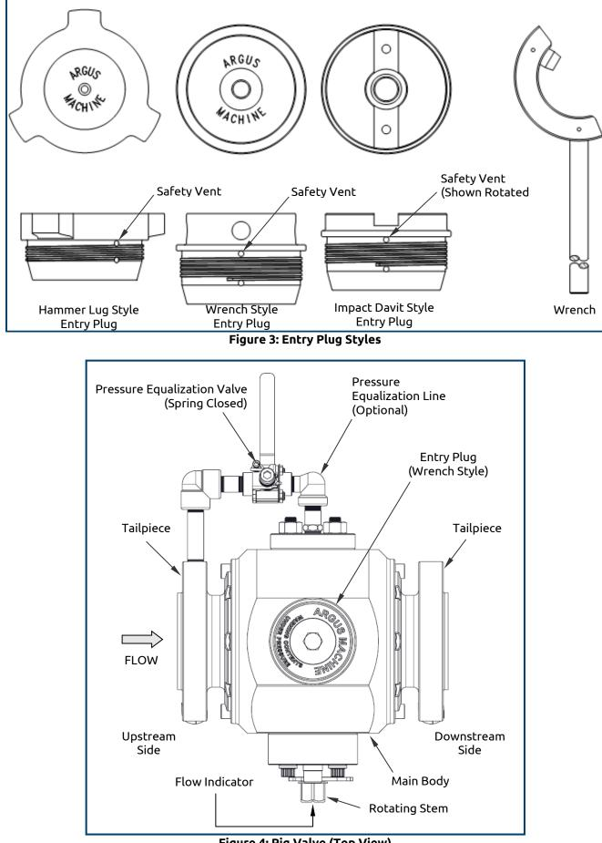
Figure 4: Pig Valve (Top View)
