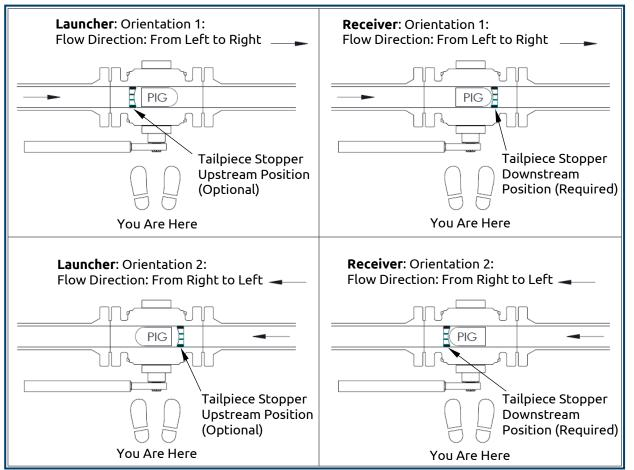
Figure 1: Pig Valve Orientation
