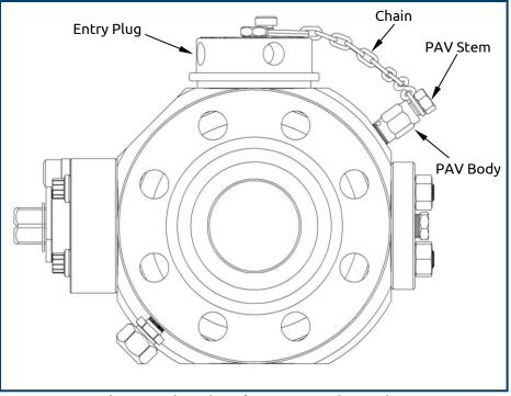
Figure 6: Pig Valve c/w Pressure Alert Valve
