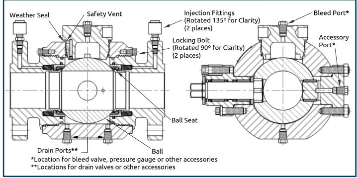
Figure 2: Pig Valve Model P
