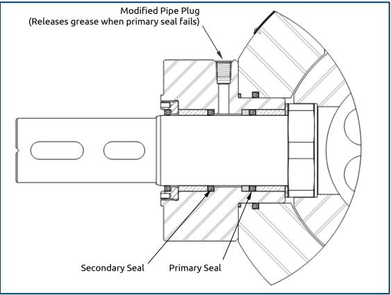
Figure 7: Stuffing Box Sub-Assembly c/w Modified Pipe Plug
