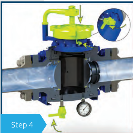
Step 4 Fully tighten the entry cap up to the alignment arrows (with the non-impact wrench), replace the pressure alert valve stem, and close all drain valves.
