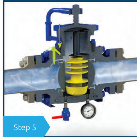
Step 5 Remove the pressure equalization valve safety pin and depress the lever to equalize the cavity pressure. The pressure gauge will increase to relative downstream pressure. Replace the pin.
