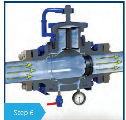
Step 6 Now in the open position, pipeline media flows through the Argus Pig Valve.
