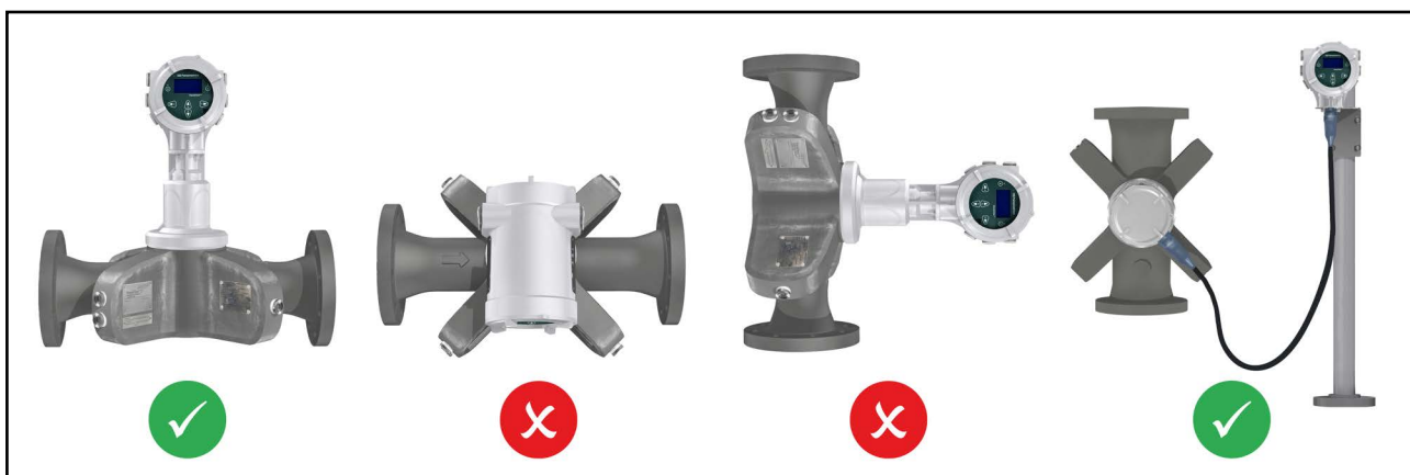
Figure 10: Transducer placement in horizontal/vertical pipes
