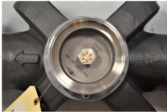
Figure 12: Connection Port to Flowcell
